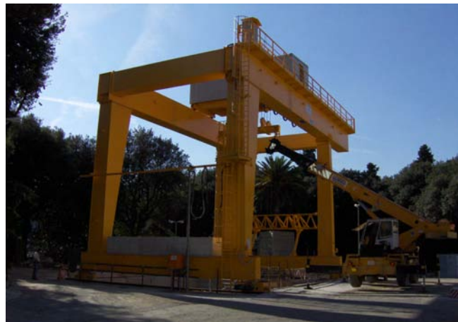
40 tons bridge crane Genova metro
