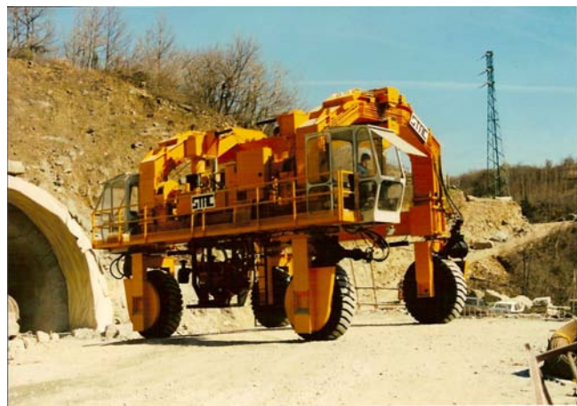
Concrete beams transport tyred trolleys
