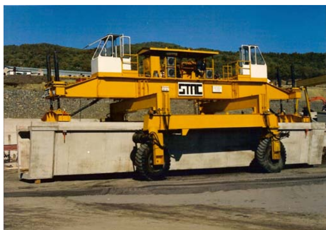
Concrete beams transport tyred trolleys
